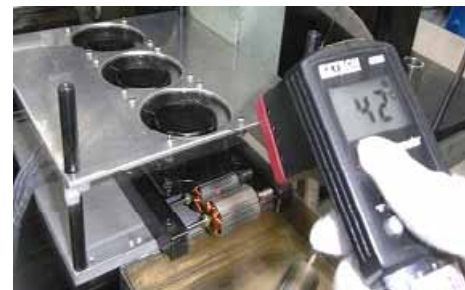
After: workpieces are cooled with an axial fan
