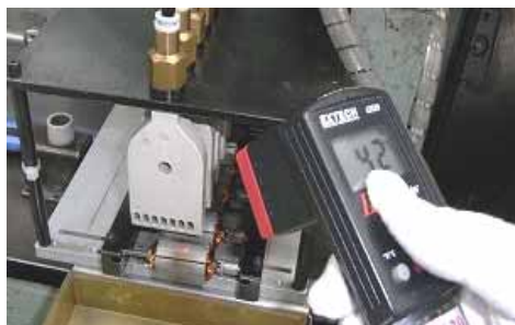
Before: workpieces were cooled with compressed air
